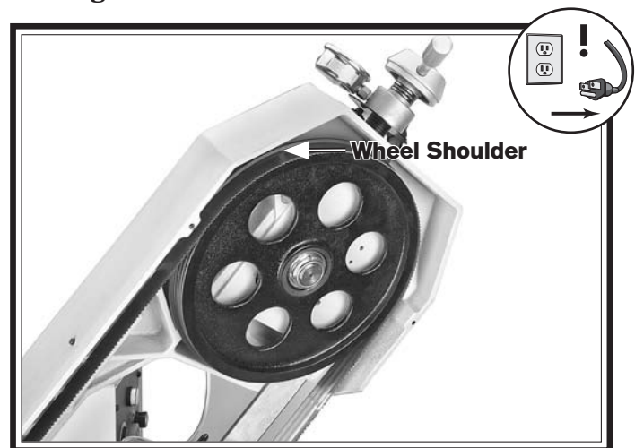
Figure 22. Typical blade/wheel position.
